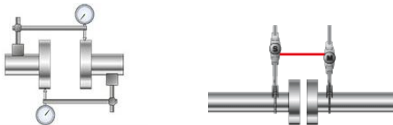
Figure 3 Dial gauge method and Laser alignment method
