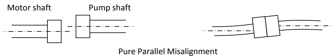
Figure 10 Shaft distortion due to parallel misalignment suggested by Piotrowski
