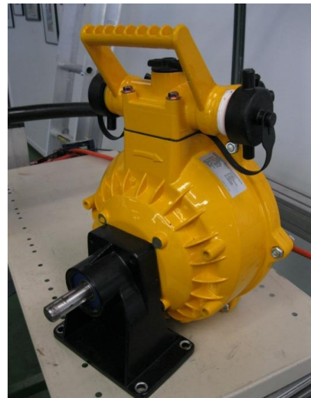
Figure 19 New pump with mechanical seal
